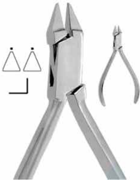
SIMZ-YM5-071 Adams Plier Adams pliers for bending wire arches and bends right angles for wires up to .022", .025 tip to beak. Length 130mm
